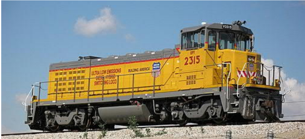
FIGURE 4-11: LOW-EMISSIONS HYBRID YARD SWITCHER LOCOMOTIVE
