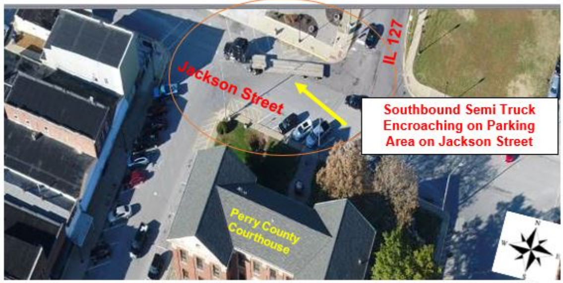
Figure 10 – Southbound Semi – Parking Spot Encroachment – Jackson Street
