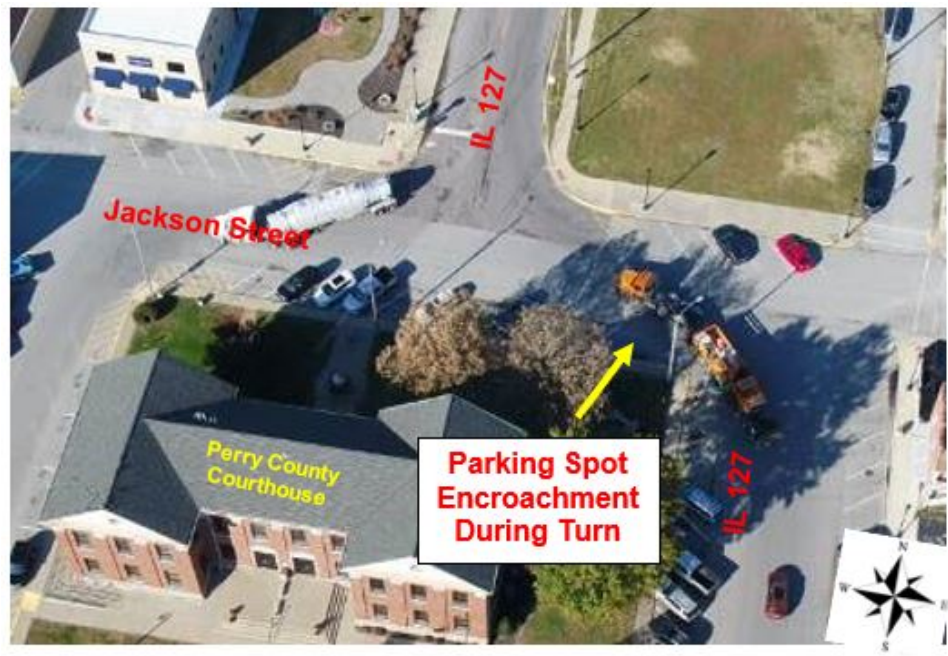
Figure 6 – Yellow Cab Truck – Parking Spot Encroachment
