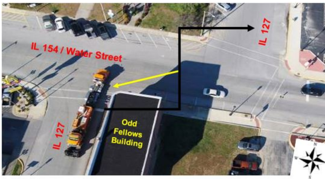
Figure 2 – Truck Encroachment – Eastbound IL 154
