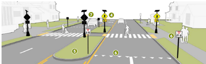
RECTANGULAR RAPID FLASHING BEACON AND CROSSING ISLAND
