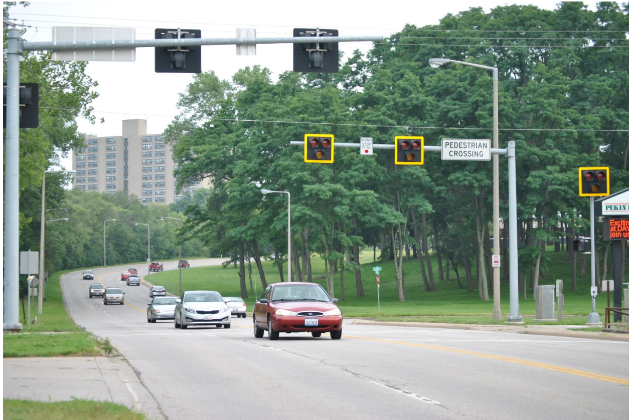
Figure 23 - PHB signal along Parkway Drive in Pekin, Illinois
