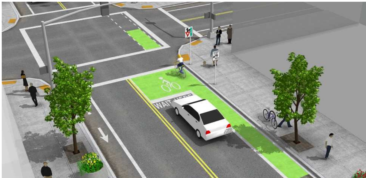
Figure 1 – Example of a bicycle box at an intersection. Image from Urban Bikeway Design Guide , by NACTO. Copyright © 2014 National Association of City Transportation Officials. Reproduced by permission of Island Press, Washington, D.C.
