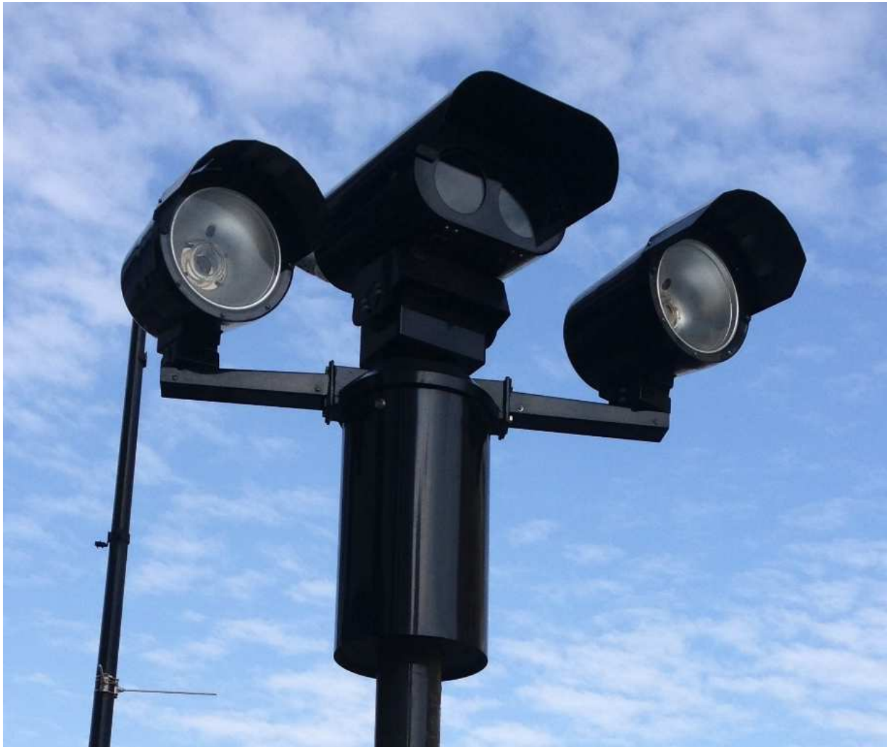
Figure 7 - Red light camera with double photo flash units along Division Street at Ashland Avenue in Chicago
