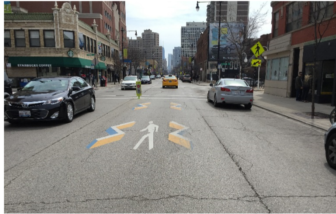
Figure 10 - 3D optical illusion pavement markings on Clark Street in Chicago
