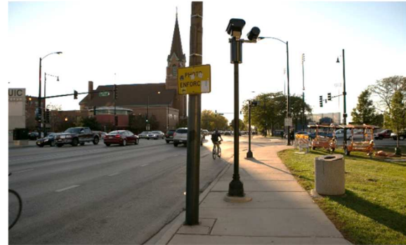
Figure 3 - Red light cameras along Roosevelt Road at Halsted Street in Chicago
