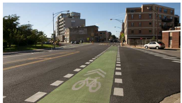
Figure 17 - Intersection crossing marking with dotted striping, colored pavement, and a shared lane marking on Milwaukee Avenue at an angled intersection in Chicago
