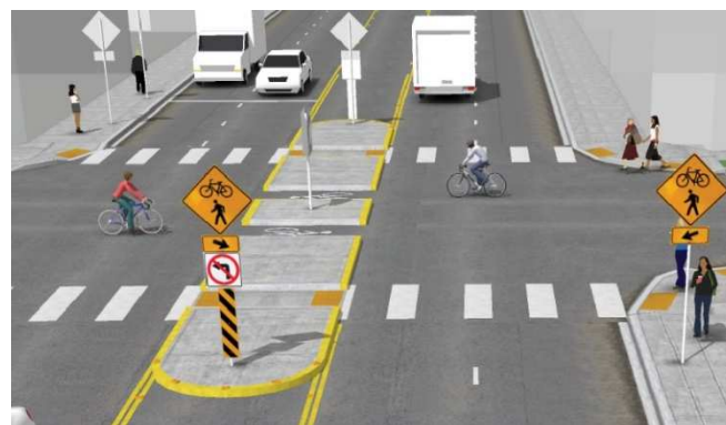
Figure 2 - Example of a median refuge island for both pedestrians and bicyclists. Image from Urban Bikeway Design Guide , by NACTO. Copyright © 2014 National Association of City Transportation Officials. Reproduced by permission of Island Press.
