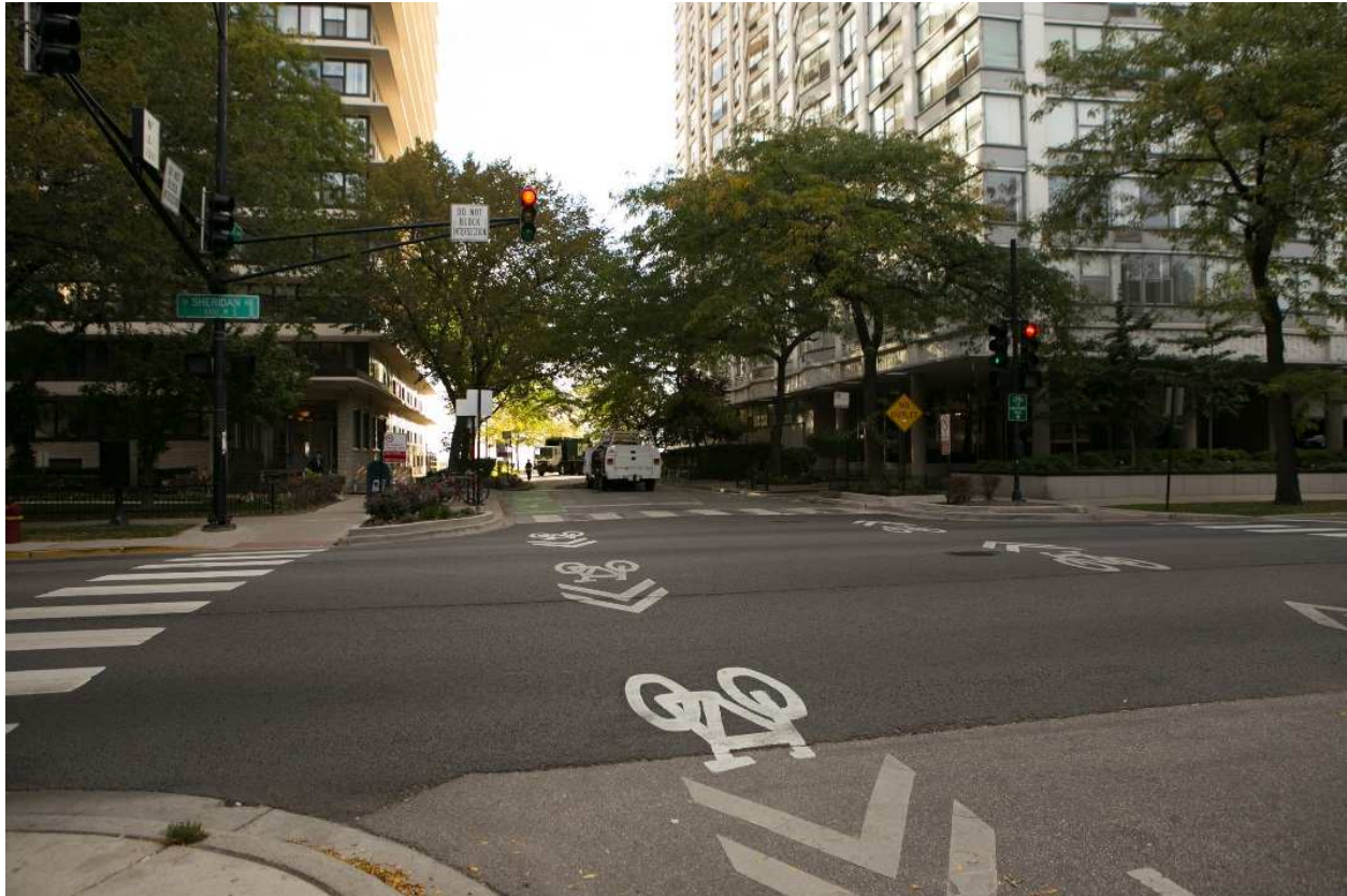
Figure 7- A bicycle boulevard crossing with intersection markings in Chicago
