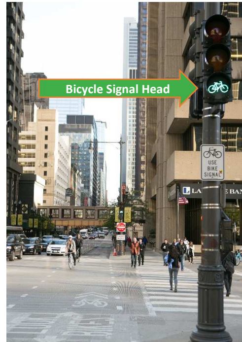
Figure 1 – Left: typical arrangements of signal sections in bicycle signal faces (MUTCD 2013). Right: Bicycle signal head on the approach side of the intersection of Dearborn Street and Wacker Drive in Chicago
