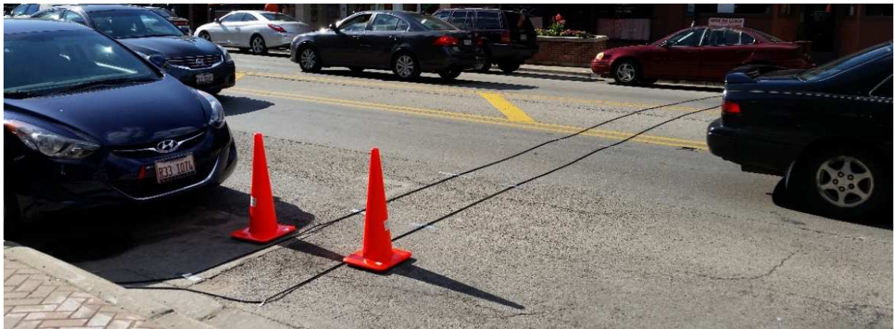
Figure 27 - Tube Set B location serving as control site and located 200 feet east of the raised crosswalk.
