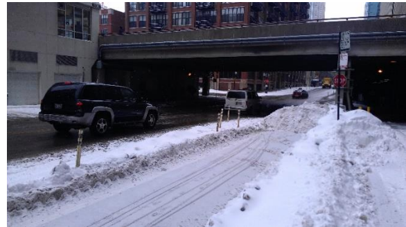
Figure 14 - Many cities experience challenges with snow removal and storage, especially in urban areas. In the image above, a nearby construction crew used a front loader to clear a separated bicycle lane in Chicago. However, the snow was piled at the end blocking the bicyclist's exit.
