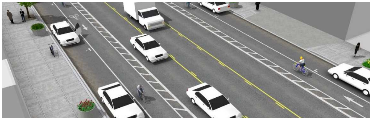
Figure 1 - Example of a buffered bicycle lane. Image from Urban Bikeway Design Guide, by NACTO. Copyright © 2014 National Association of City Transportation Officials. Reproduced by permission of Island Press, Washington, D.C.
