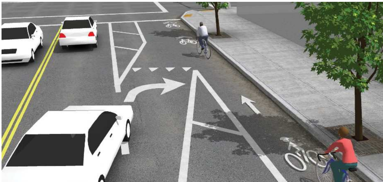
Figure 1 - Mixing zone with "shark's teeth" yield markings and shared lane markings. Image from Urban Bikeway Design Guide, by NACTO. Copyright © 2014 National Association of City Transportation Officials. Reproduced by permission of Island Press, Washington, D.C.
