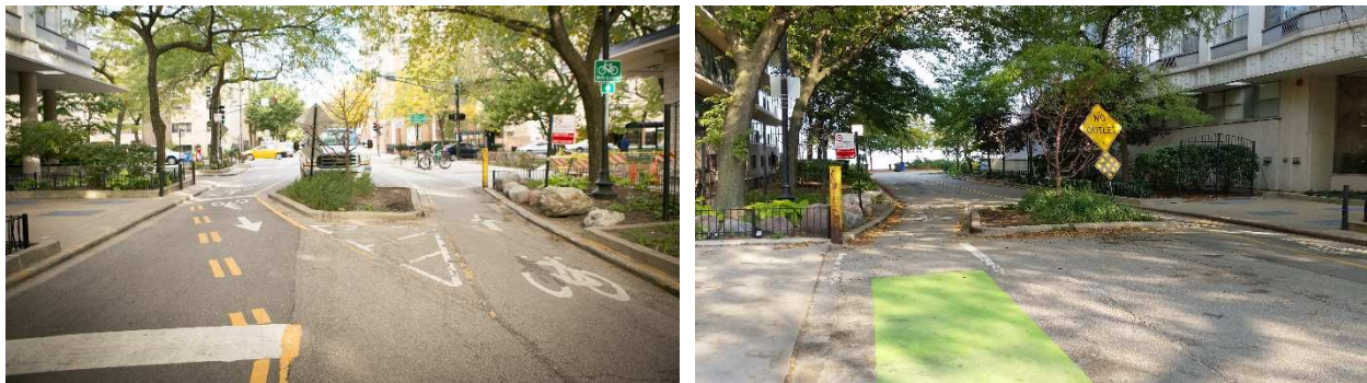
Figure 11 - Example of a cul-de-sac type with restricted openings only for bicyclists on either side of the landscaped median. The cut through connects a bicycle boulevard to the shared use Lake Front Trail in Chicago.
