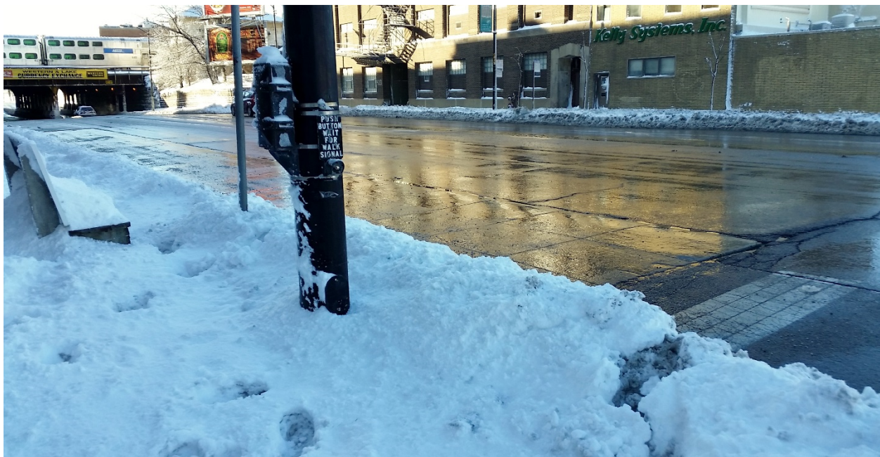
Figure 12 - Difficult to access pedestrian activation button in Chicago
