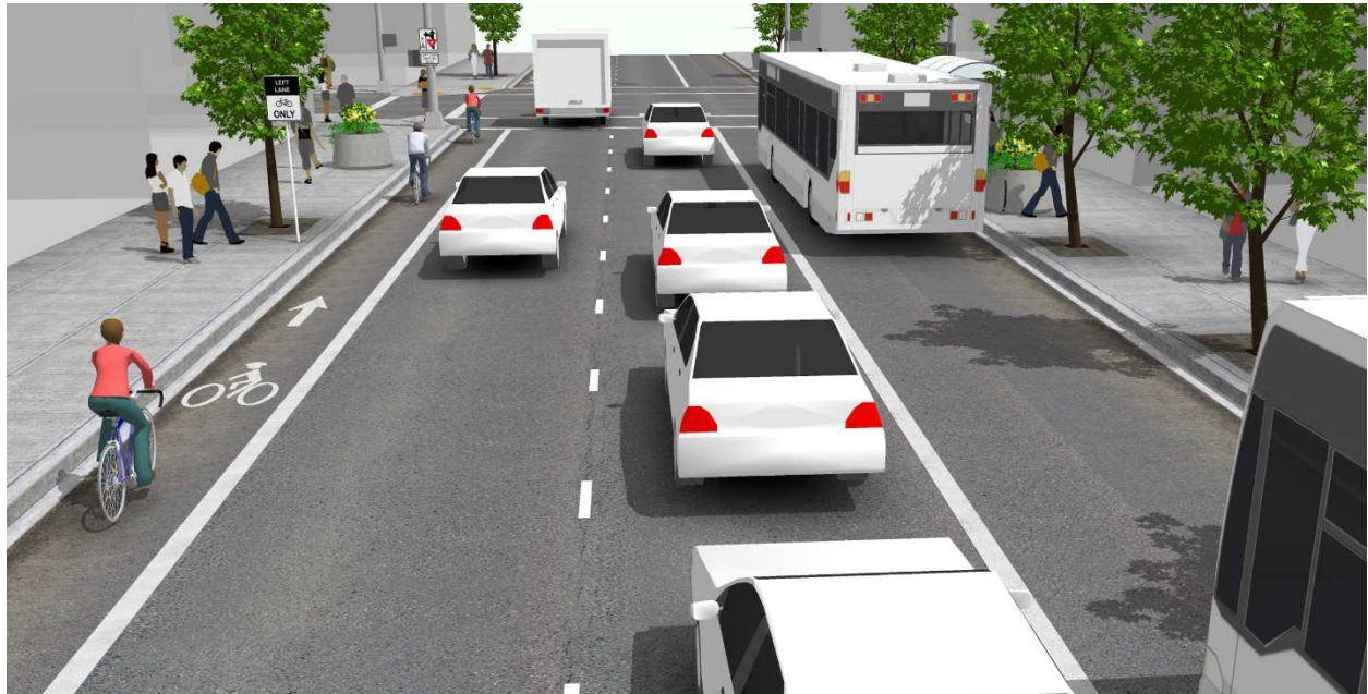
Figure 2 – Left-side bicycle lane. Image from Urban Bikeway Design Guide , by NACTO. Copyright © 2014 National Association of City Transportation Officials. Reproduced by permission of Island Press, Washington, D.C.
