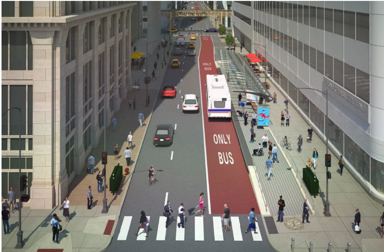
Figure 4 - A rendering of a proposed bus bulb in Chicago as part of Chicago's LoopLink project. Image courtesy of CDOT. Reprinted with permission.
