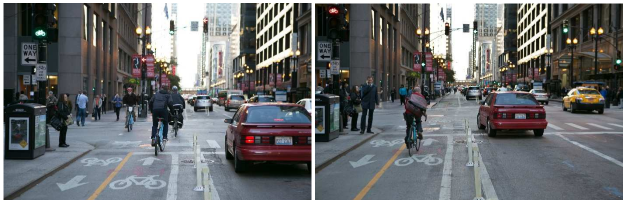
Figure 8 - Left: bicyclists have the green light and continue straight. Right: the turning motorist has the green light while the bicyclist stops on red.
