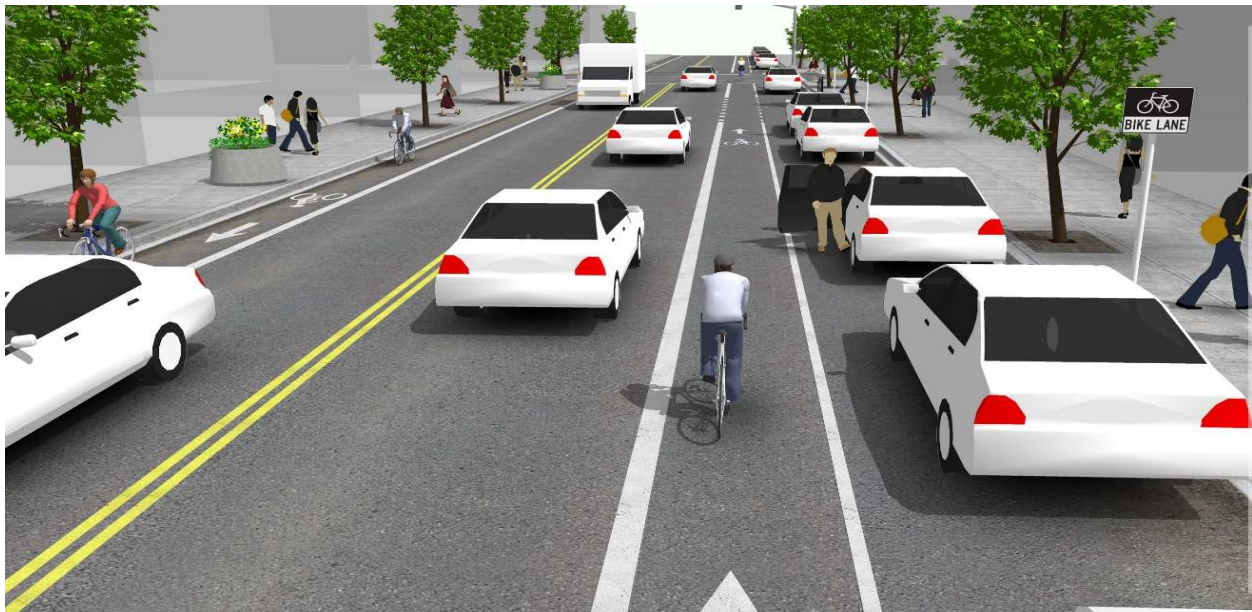
Figure 1 - Example of a conventional bicycle lane. Image from Urban Bikeway Design Guide , by NACTO. Copyright © 2014 National Association of City Transportation Officials. Reproduced by permission of Island Press, Washington, D.C.
