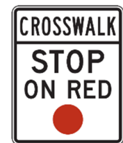
Figure 5 - R10-23 sign, "Crosswalk, Stop on Red"
