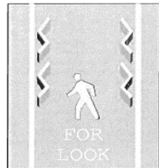
Figure 4 - Layout of pavement markings along Clark Street approaching the intersection with Deming Place in Chicago
