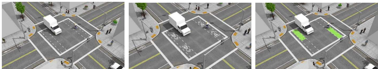
Figure 7 - Various bicycle pavement markings through an intersection. Images from Urban Bikeway Design Guide , by NACTO. Copyright © 2014 National Association of City Transportation Officials. Reproduced by permission of Island Press, Washington, D.C.
