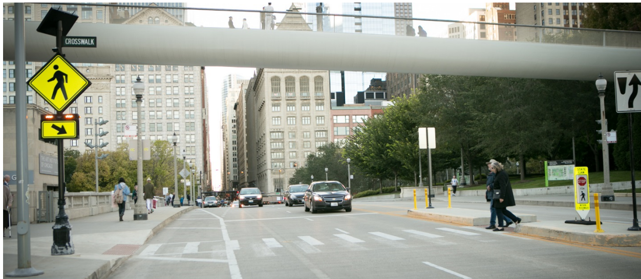
Figure 1 – Midblock RRFB located on Madison Street between Millennium Park and the Art Institute in Chicago
