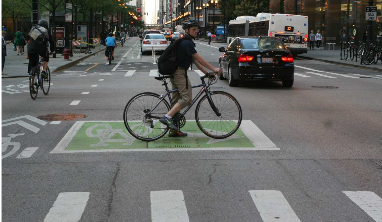
Figure 48 – Bicyclist making a turn from a two-way SBL and positioned within the two-stage turn box on Dearborn Street in Chicago
