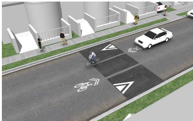
Figure 6 – Speed humps, a potential speed reduction treatment, can contain cutouts that do not impact bicyclist speed or comfort. Image from Urban Bikeway Design Guide, by NACTO. Copyright © 2014 National Association of City Transportation Officials. Reproduced by permission of Island Press.
