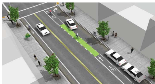
Figure 27 – Example lateral shift. Image from Urban Bikeway Design Guide, by NACTO. Copyright © 2014 National Association of City Transportation Officials. Reproduced by permission of Island Press, Washington, D.C.
