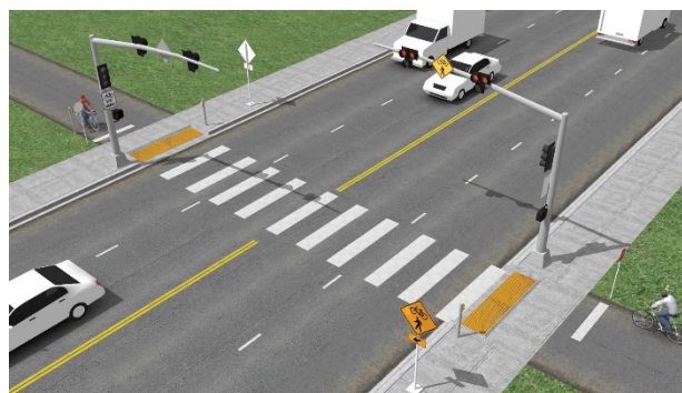
Figure 8 - Example of a PHB and a midblock shared use path crossing. Image from Urban Bikeway Design Guide, by NACTO. Copyright © 2014 National Association of City Transportation Officials. Reproduced by permission of Island Press, Washington, D.C.
