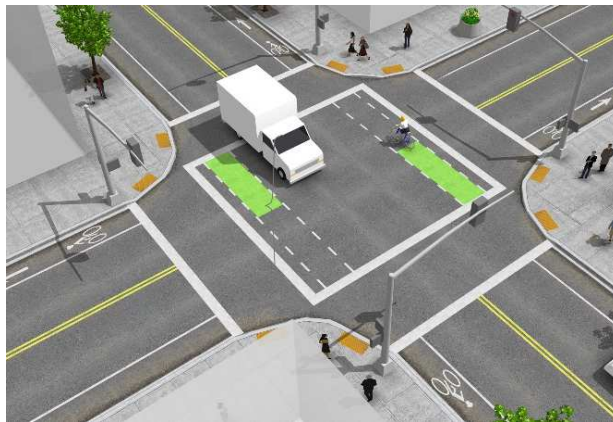
Figure 53 - Pavement markings at intersection. Image from Urban Bikeway Design Guide , by NACTO. Copyright © 2014 National Association of City Transportation Officials. Reproduced by permission of Island Press, Washington, D.C.
