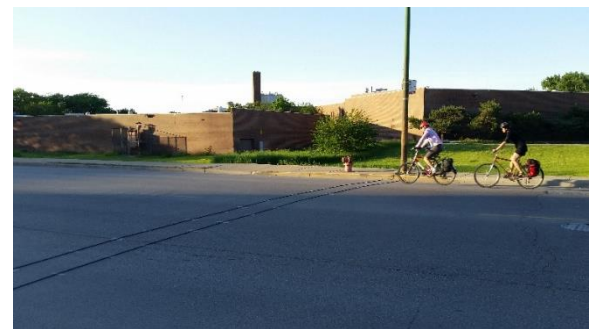
Figure 32 - Pneumatic tubes collecting short term bicycle counts on Clybourn Street in Chicago
