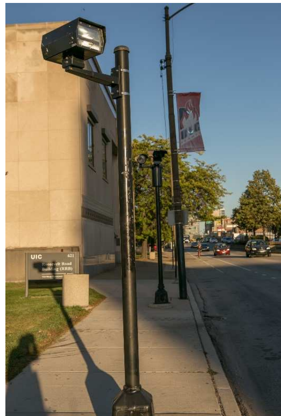
Figure 1 – Red light cameras along Roosevelt Road at Halsted Street in Chicago
