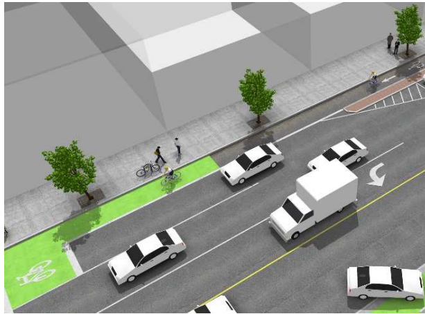
Figure 52 - Cycle track transition to bicycle lane and bicycle box. Image from Urban Bikeway Design Guide , by NACTO. Copyright © 2014 National Association of City Transportation Officials. Reproduced by permission of Island Press, Washington, D.C.
