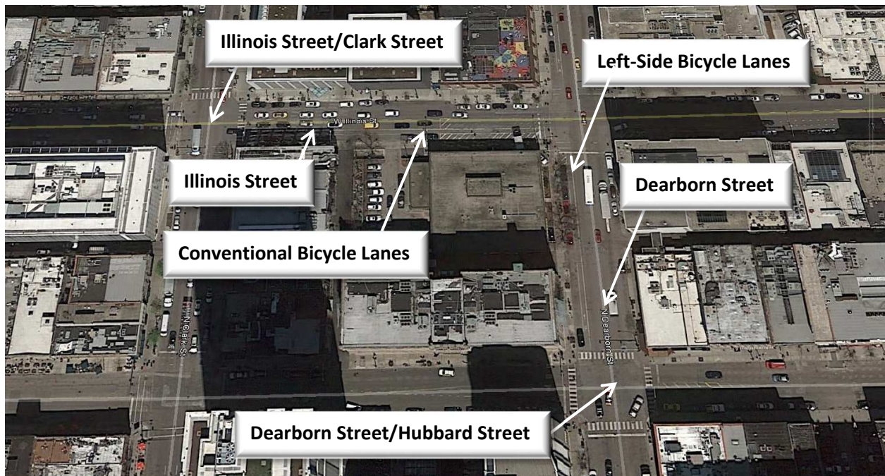
Figure 20 - Left-side bicycle lane along Dearborn Street at the intersection with Hubbard Street
