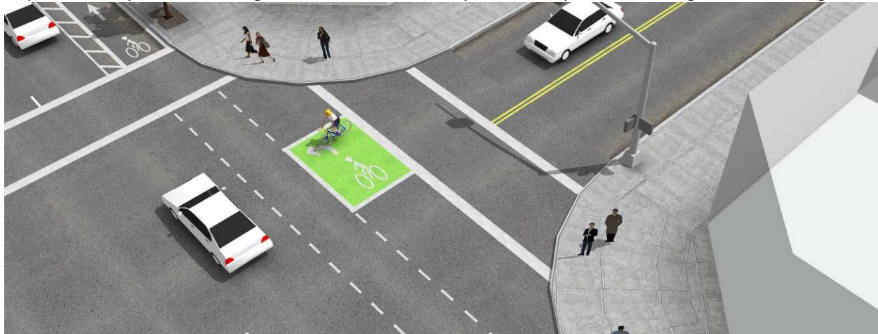
Figure 5 - Two-stage turn box diagram on a one-way separated bicycle lane. Image from Urban Bikeway Design Guide, by NACTO. Copyright © 2014 National Association of City Transportation Officials. Reproduced by permission of Island Press, Washington, D.C.
