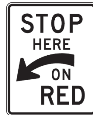
Figure 2 - MUTCD signage (R10-6a) instructing motorists to stop at the stop bar and discourage encroachment on the bicycle box.
