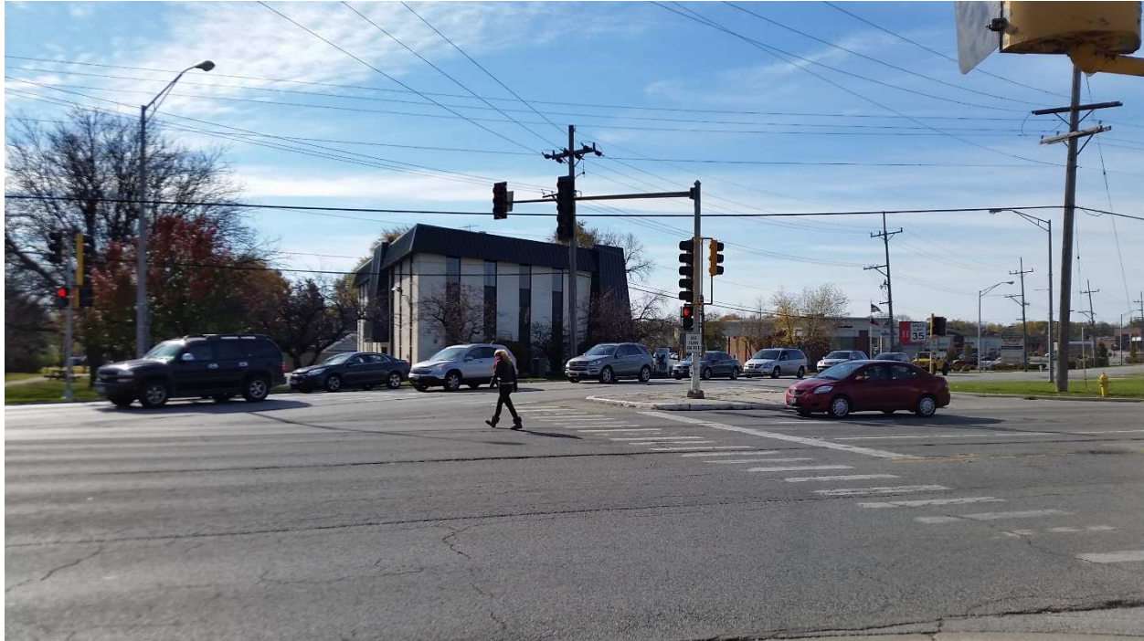
Figure 10 - Pedestrian walking outside the crosswalk due to a stopped motorist encroaching on the intersection. Located at the intersection of 55th Street and Plainfield Road in Countryside, Illinois that has an exclusive pedestrian phase.
