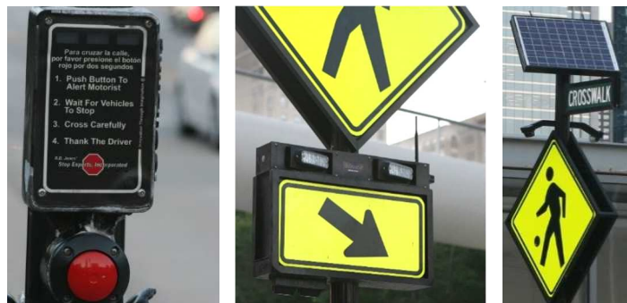
Figure 2 - Features of the RRFB. From left to right: pedestrian activated push button, RRFB, and solar panel.
