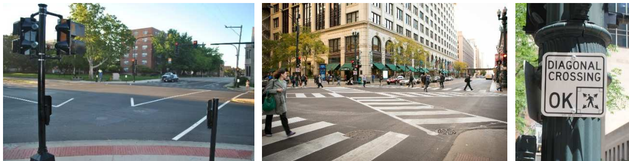
Figure 1 - Examples of exclusive pedestrian phase crossings and signage.
