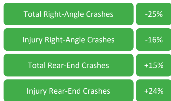
Figure 4 - Percent change in crashes before and after installation of red light cameras. Source: FHWA.
