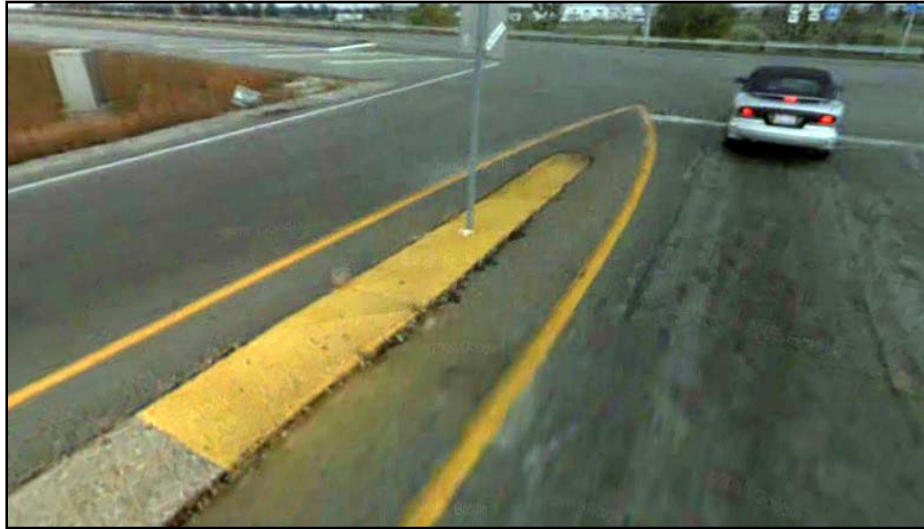
Figure 2-14. Painted island between exit and entrance ramps (Morena and Ault 2013).
