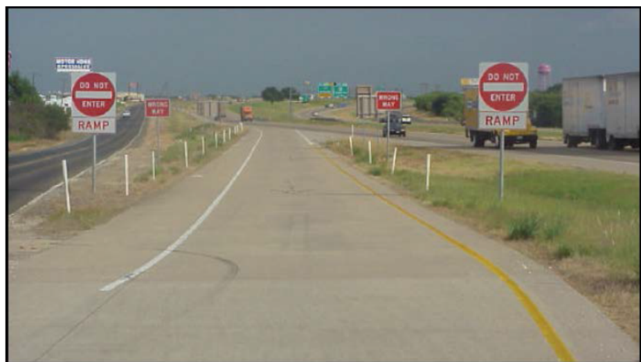
Figure 2-2. Supplemental RAMP placards on DNE signs (Cooner et al. 2004).
