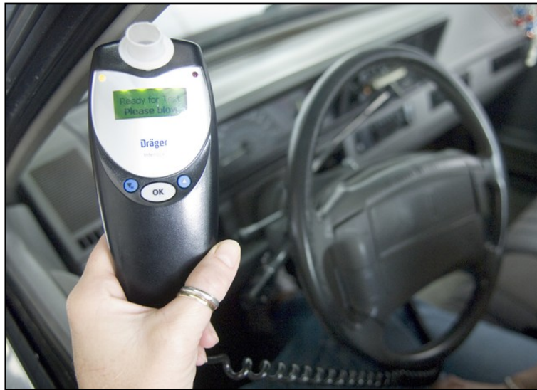
Figure 4-12. Ignition interlock system detects the alcohol content in a driver's breath before the engine can be started (CNRL 2012).
