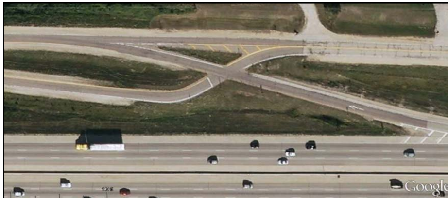
Figure 3-17. Scissors channelization (Image: Google Earth).
