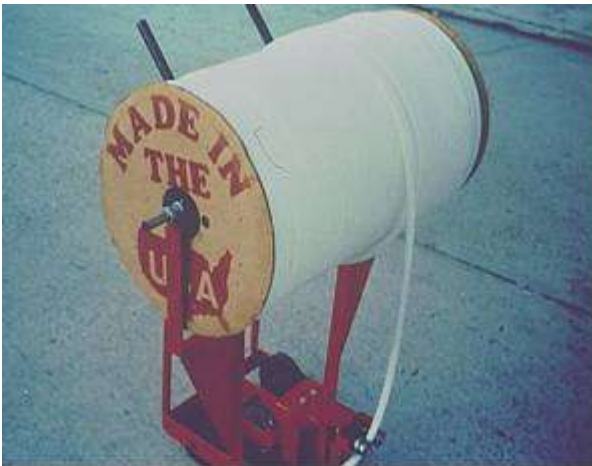
Step 3. Backer rod installation. Backer rod can be used to control the depth of the sealant in the crack.
