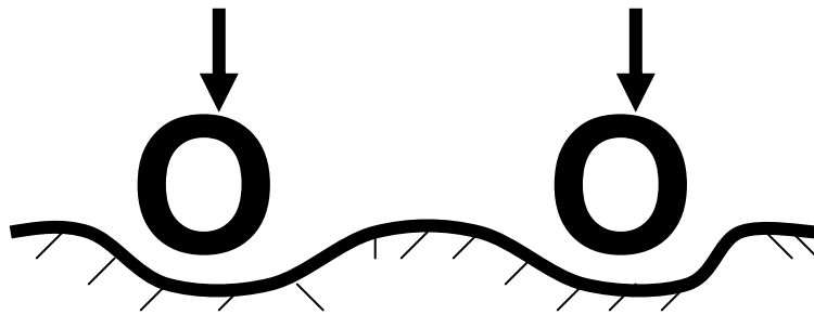
Figure 1. Resilient (rebound) deflections of silty soils under wheel loads makes compaction of pavement layers difficult.
