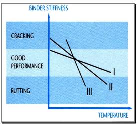
Figure 1: Temperature Responses of Different Binder Materials
