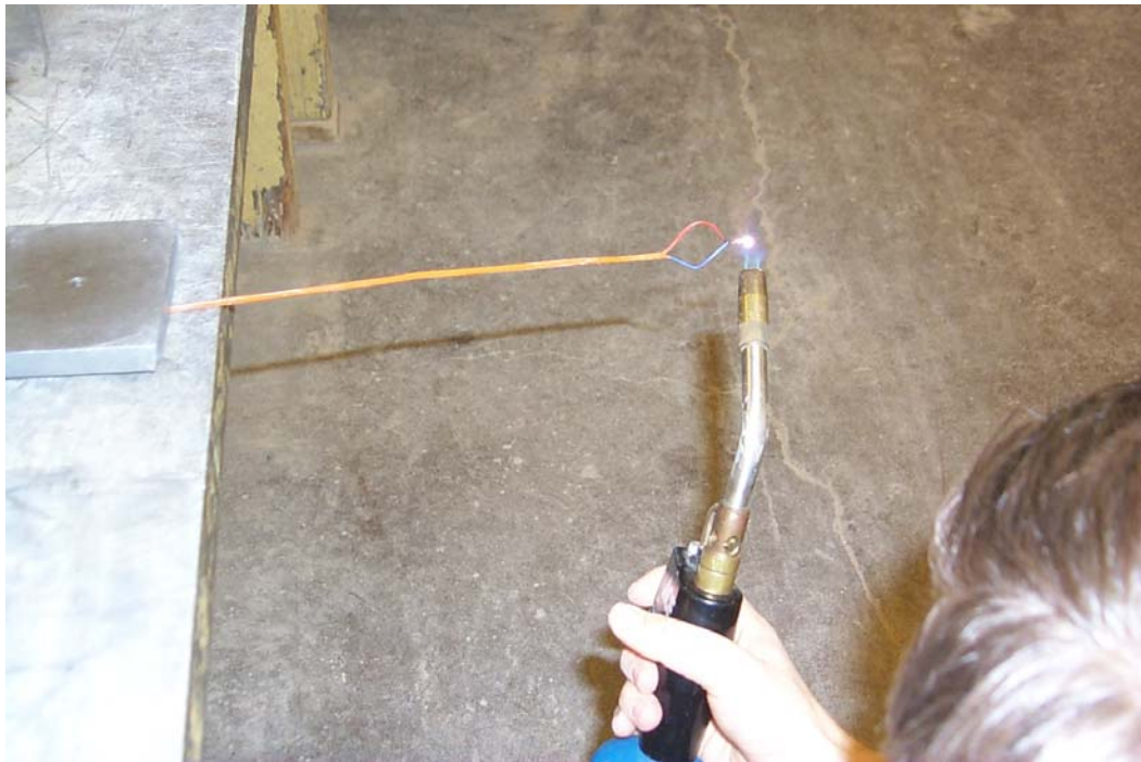
Figure 1. Soldering the wires.
