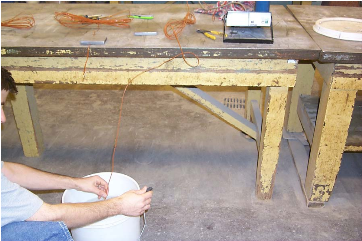
Figure 2. Testing the soldered thermocouple.
