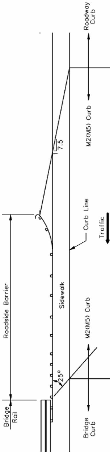
USE OF ROADSIDE BARRIER WITH M2 (M5) CURB
