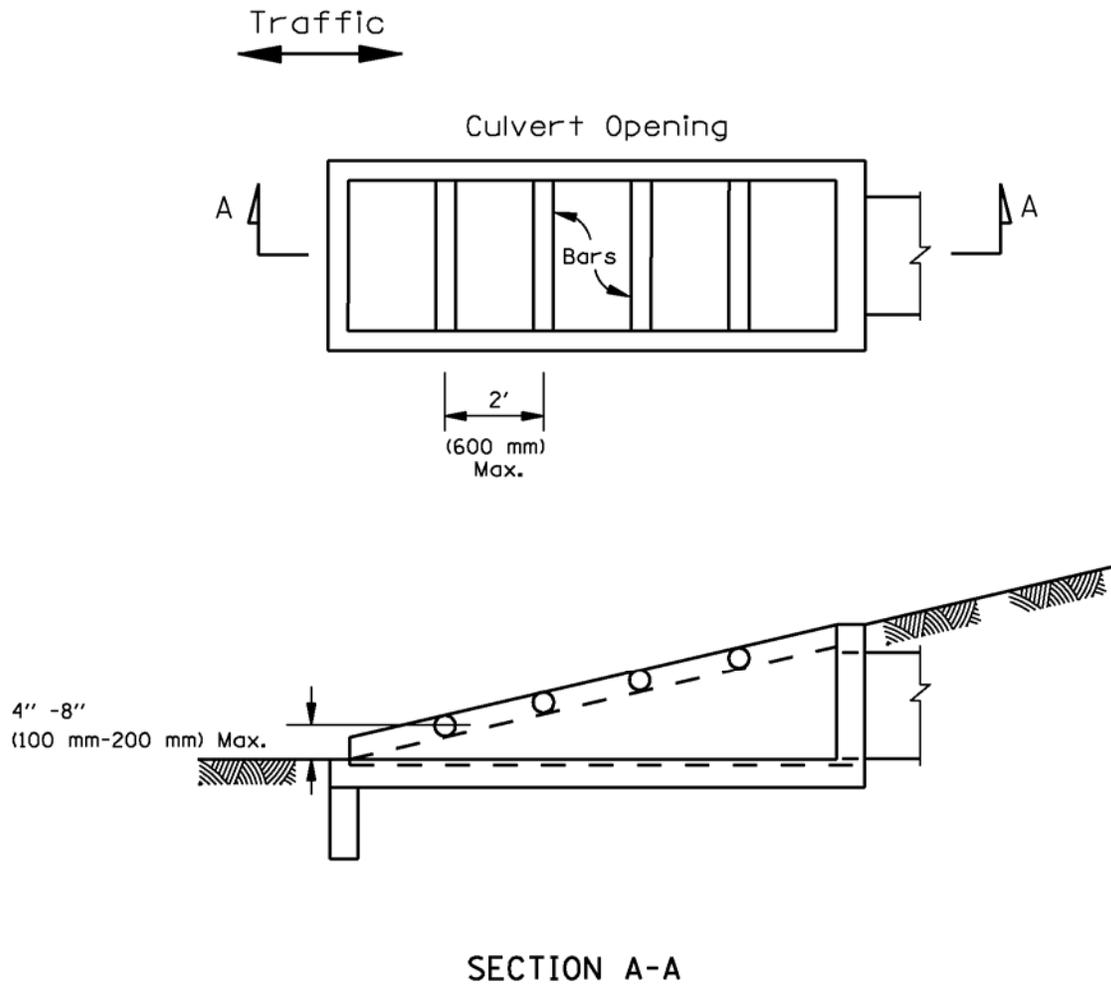
GRATE PROTECTION FOR PARALLEL DRAINAGE STRUCTURES
