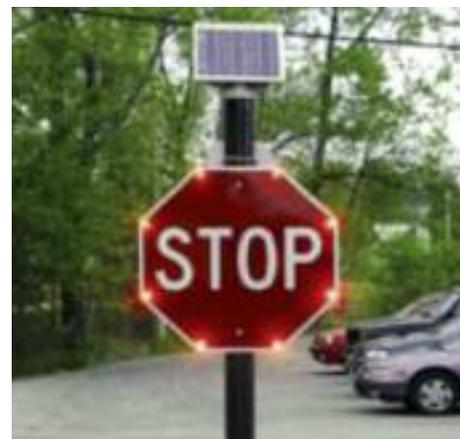
Example of stop sign with embedded LEDs and solar unit.
