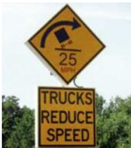
LEDs are embedded in the symbols and lettering on this truck warning sign.
