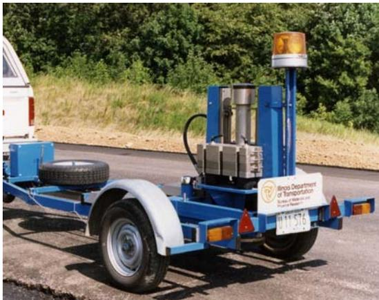
**Figure 1: Falling Weight Deflectometer**
