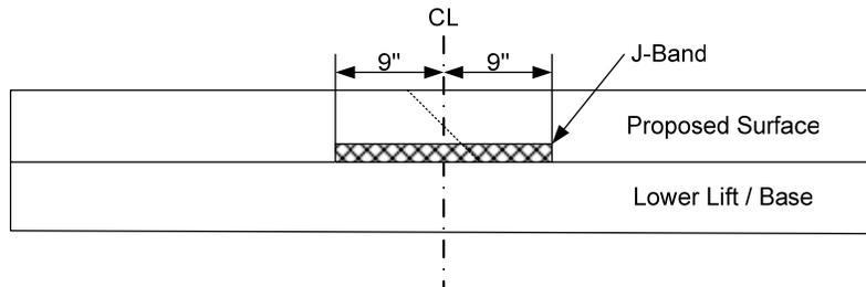
Figure 2: J-Band<sup>®</sup> Placement
