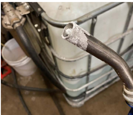
Urea from DEF can build up on nozzles in the form of crystals. These crystals can then contaminate the DEF tank.
