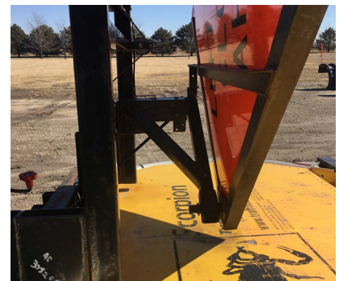
The holder was designed to attach to the arrow board frame only, keeping the TMA intact.
