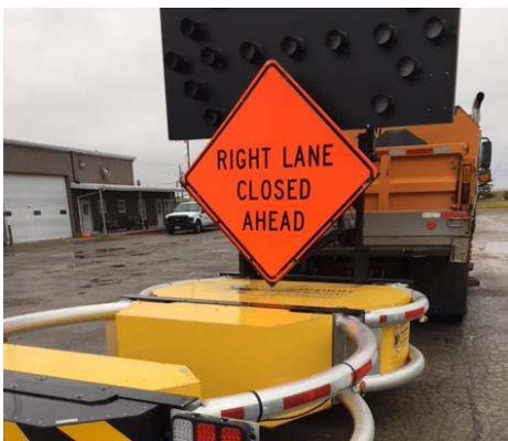
Signs displayed on TMAs in work zones provide valuable traffic safety controls that help keep workers and motorists safe.
