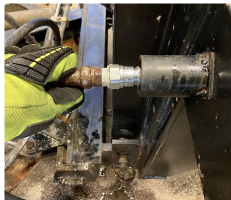
The depressurization chamber is a simple attachment that safely eliminates hydraulic pressure in a controlled manner.
