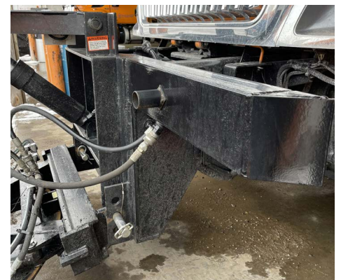
The chamber is bolted to the bumper near hydraulic fittings for ease of use.
