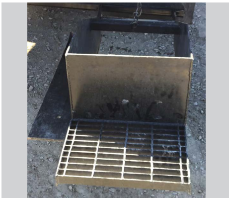
The aggregate shoulder spreader box was created using surplus materials found at the yard.
