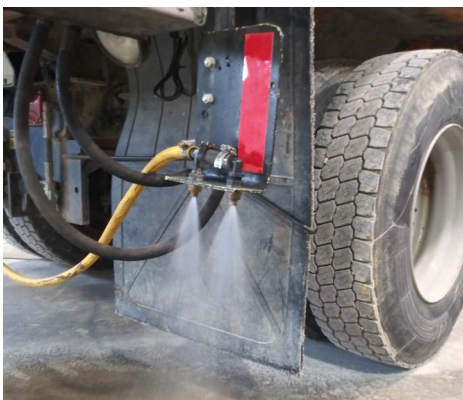
The system safely applies brine to the white line at a fraction of the cost of dual spinners.
