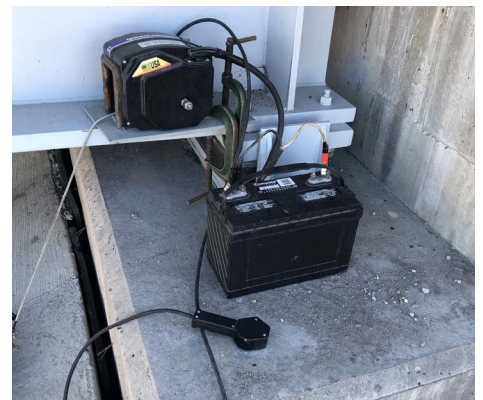
A power winch easily gets the sled where it needs to go.
