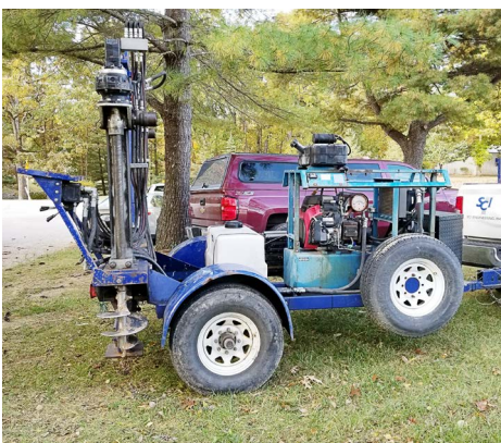
The CPT equipment has a smaller footprint and can be towed by department vehicles.
