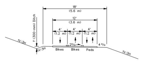
TYPICAL SHARED USE PATH FOR SUBSTANTIAL SHARED USE (More Than 300 Users in Peak Hour, Striping is Optional)
