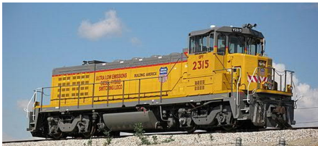
FIGURE 4-11: LOW-EMISSIONS HYBRID YARD SWITCHER LOCOMOTIVE
