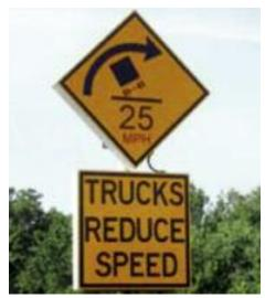
LEDs are embedded in the symbols and lettering on this truck warning sign.
